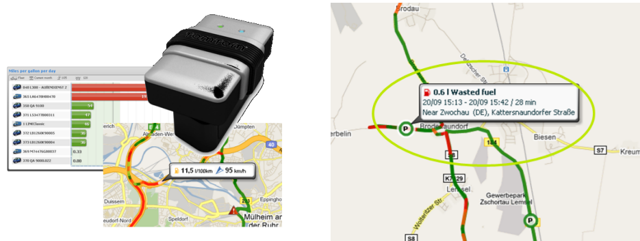
Figure 3: TomTom Business Solution's ecoPLUS product, an accessory connecting to a vehicle's onboard diagnostic connector to deliver real-time fuel consumption and CO 2 emissions to a web-based server application.
